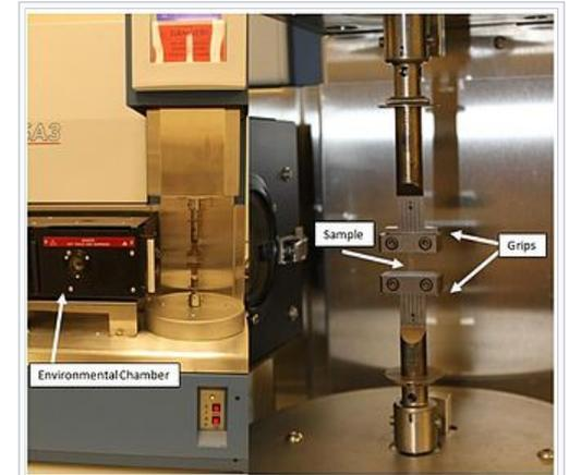
Figure 1. A typical DMA tester with grips to hold sample and environmental chamber to provide different temperature conditions. A sample is mounted on the grips and the environmental chamber can slide over to enclose the sample.
