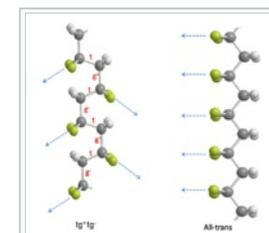
Figure 6: Schematic description of two most common conformations of PVDF, the left one is tg<sup>+</sup>tg<sup>-</sup> and the right one is all trans, the yellow sphere represents fluorine atom, the white sphere represents hydrogen atom and the grey sphere represents the carbon atom.
