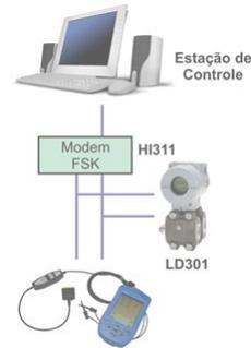
Figure 36 - HART point to point connection
