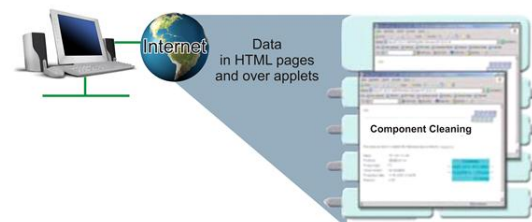
Figura 15 – The access to PROFINet data information can be done through the standard WEB services.
