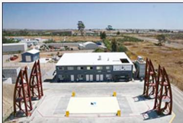
The Large High-Performance Outdoor Shake Table can handle structures weighing up to 2,200 tons without height restrictions. The table's powerful hydraulic actuators can move at up to 6 feet per second, creating realistic simulations of the most devastating earthquakes ever recorded.
