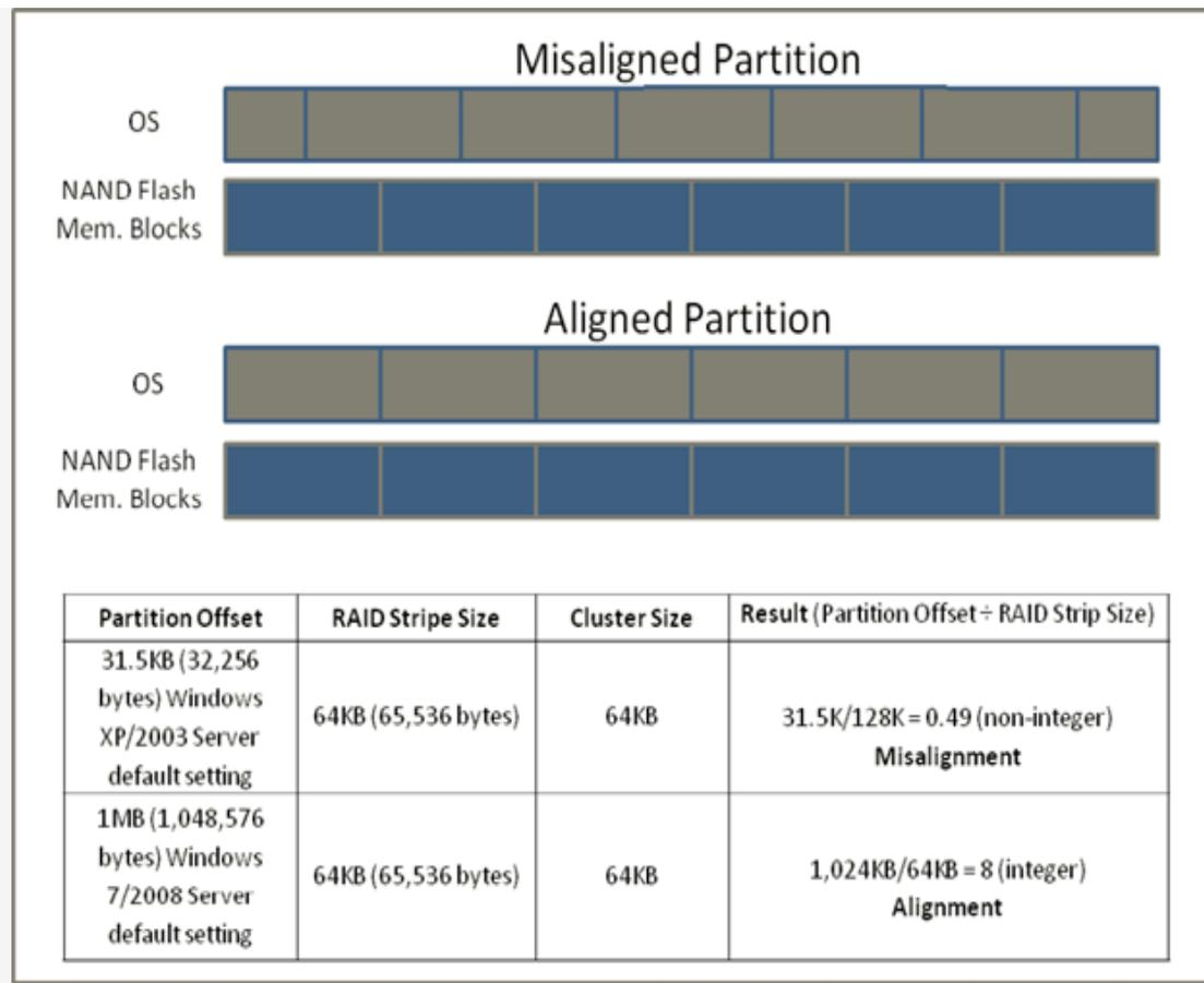
When choosing a partition starting offset, SMART Modular recommends system integrators to correlate the partition offset with the RAID stripe size and cluster size to achieve the optimal SSD I/O performance. The figure shows an example of a misaligned partition offset and an example of an aligned partition offset for Windows Server.”
